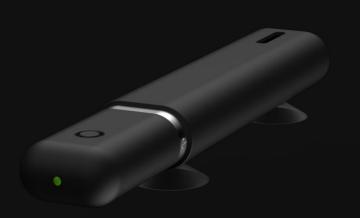
Special case for XS designed for an HACCP client in order to monitor restaurant fridges temperatures. XS firmware has also been redesigned in order to meet clients constraints.
